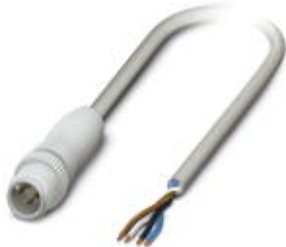
Sensor/Actuator cable, 4-position, PP-EPDM halogen-free, Gray RAL 7035, Plug straight M12, A-coded, on Free cable end, Cable length: 3 m, Hygienic design, with plastic knurl
