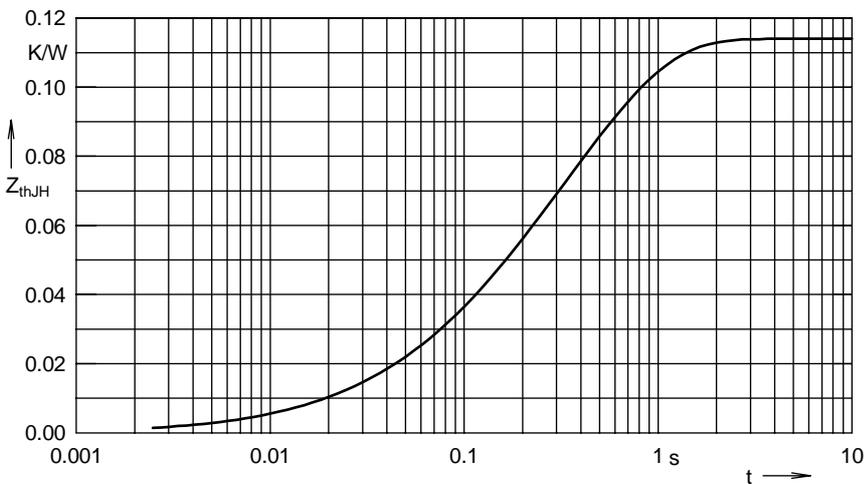
Fig. 7 Transient thermal impedance junction to heatsink
