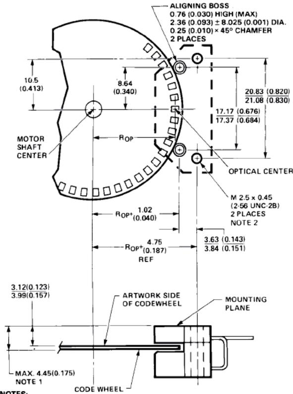
Figure 2. Mounting Plane Side A.
