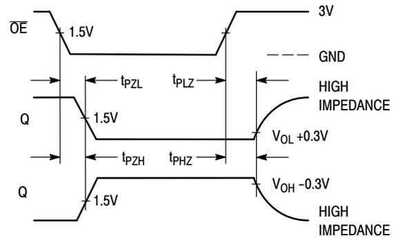
Figure 4. Switching Waveform
