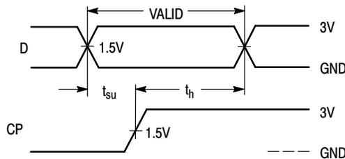
Figure 5. Switching Waveform
