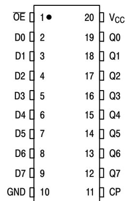
Figure 2. Pin Assignment
