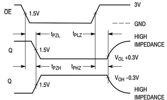
Figure 4. Switching Waveform
