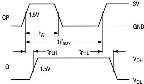
Figure 3. Switching Waveform
