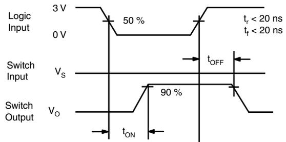
**Figure 1. Single Supply Switching Time**
