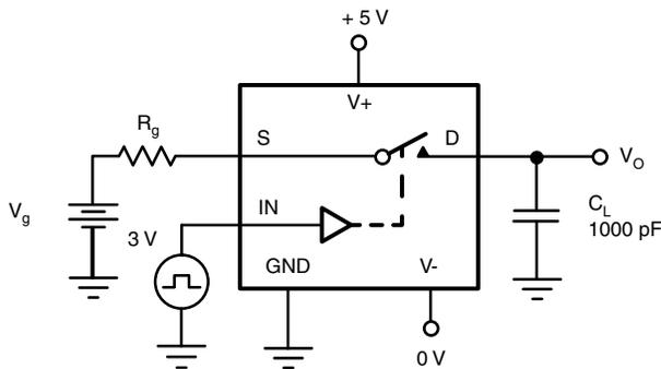
**Figure 3. Charge Injection**
