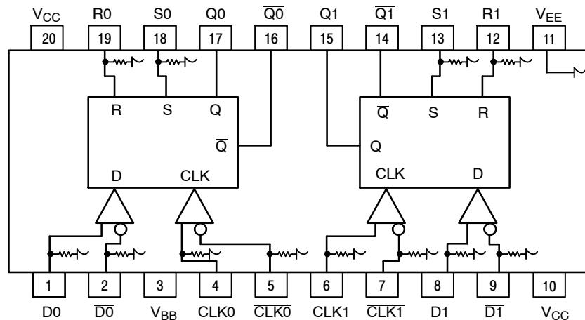
Warning: All V<sub>CC</sub> and V<sub>EE</sub> pins must be externally connected to Power Supply to guarantee proper operation.
