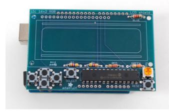
Place the shield right on top. It should fit perfectly where all the short ends of the header fit into the holes of the shield.
