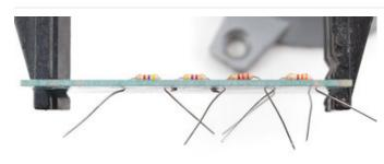
Make sure the resistors all sit nice and flat against the PCB.
