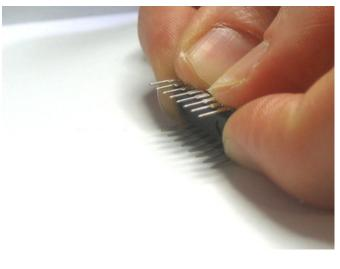
We're nearly done! Now we will place the I2C port expander chip. Double check that it has the **MCP23017-E/SP** marking on it. This is a 16-pin expander chip, that uses the i2c bus. That means you can send it commands using the i2c pins on an Arduino and control 16 more digital pins! 5 of those pins go to the buttons, 6 go to the LCD control and 3 are used for the backlight (the remaining 2 are unused).
