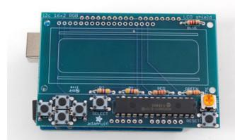
Place the shield right on top. It should fit perfectly where all the short ends of the header fit into the holes of the shield.
