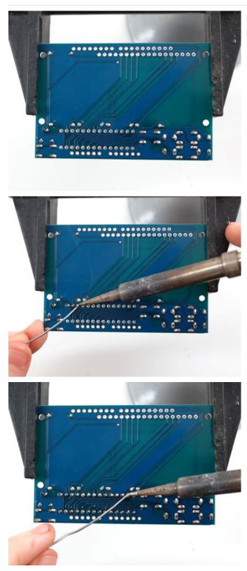
Flip over the PCB and solder in the three legs of the potentiometer and then all 28 pins of the port expander.
