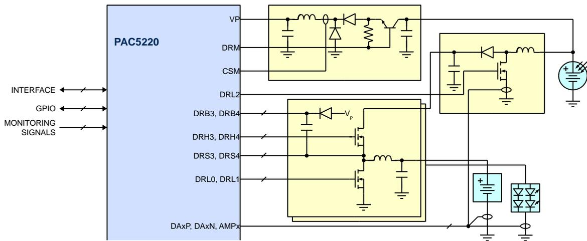
Figure 21-3 WPC type A11 Wireless Power Transmitter Using PAC5220 (Simplified Diagram)
