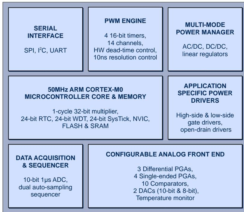
The PAC5220 is available in a 56-pin, 8mmx8mm TQFN package. The PAC family includes a range of part numbers optimized to work with different targeted primary applications.
