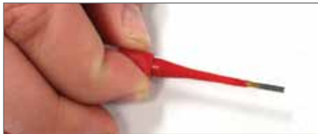
Plastic tool with contact in proper position.
