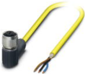
Sensor/Actuator cable, 3-position, PVC, Yellow RAL 1021, shielded, Free cable end, on Socket angled M12-SPEEDCON, A-coded, Cable length: 10 m
