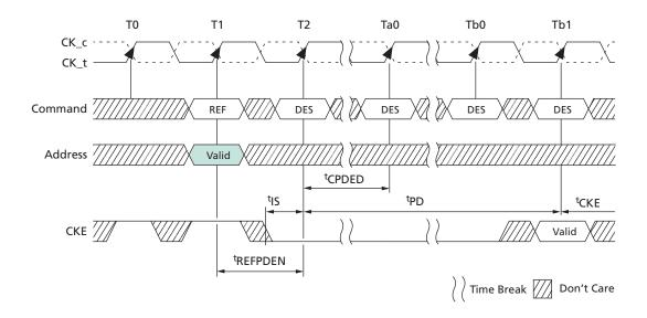
**Figure 99: Active Command to Power-Down Entry**
