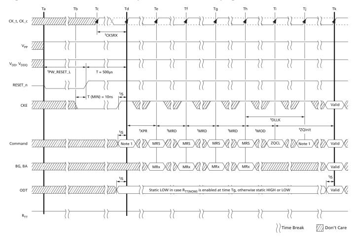
Figure 15: RESET and Initialization Sequence at Power-On Ramping
