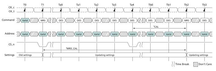
Note: 1. Command address latency mode is enabled at T1.
