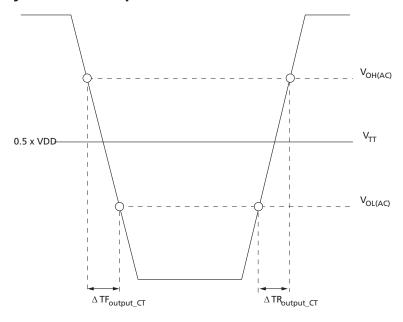
**Table 120: Connectivity Test Mode Output Slew Rate**
