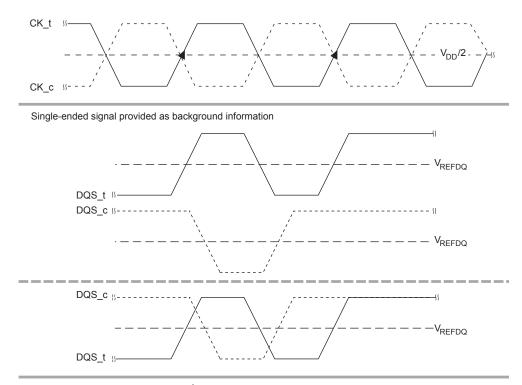
Resulting differential signal relevant for \$\$^tWPST\$ specification
