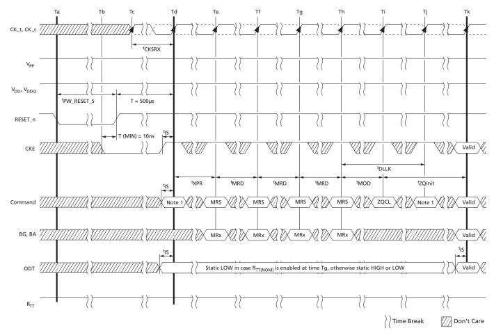
**Figure 16: RESET Procedure at Power Stable Condition**
