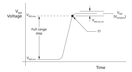
Figure 72: V<sub>REF</sub> Full Step: From V<sub>REF,max</sub> to V<sub>REF,min</sub>Case
