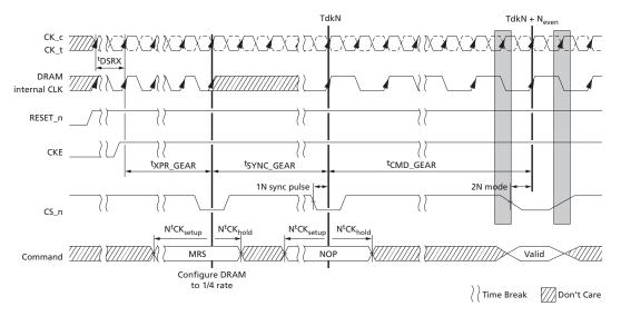
Figure 45: Clock Mode Change After Exiting Self Refresh
