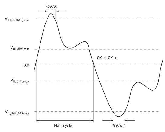
Notes: 1. Differential signal rising edge from V<sub>IL,diff,max</sub> to V<sub>IH,diff(AC)min</sub> must be monotonic slope.
