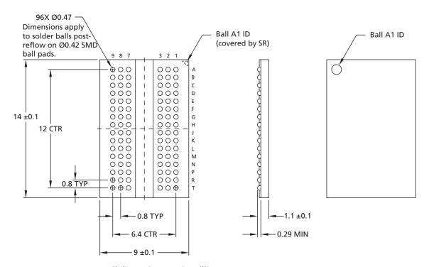
2. Solder ball material: SAC302 (Pb-free 96.8% Sn, 3% Ag, 0.3% Cu).
