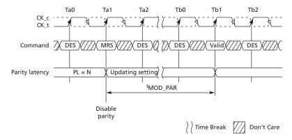
Note: 1.  ${}^{t}MOD_{PAR} = {}^{t}MOD + N$ ; where N is the programmed parity latency.
