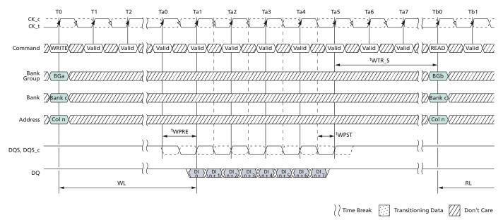
Note: 1. tWTR\_S: delay from start of internal write transaction to internal READ command to a different bank group.
