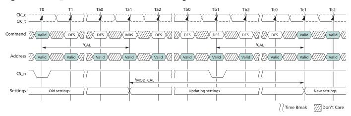
Note: 1. MRS at Ta1 may or may not modify CAL, <sup>t</sup>MOD\_CAL is computed based on new <sup>t</sup>CAL setting if modified.
