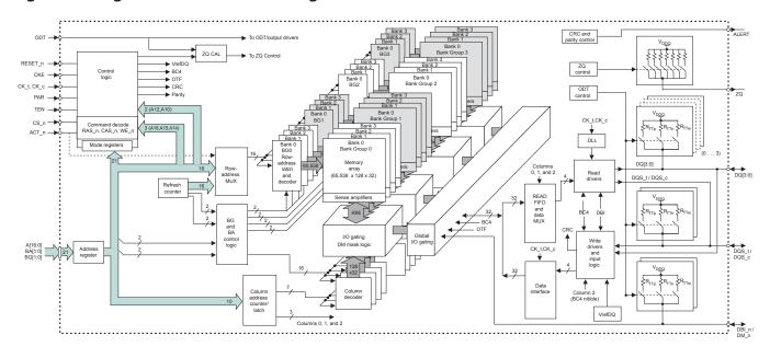
Figure 3: 512 Meg x 8 Functional Block Diagram
