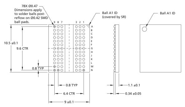
2. Solder ball material: SAC302 (Pb-free 96.8% Sn, 3% Ag, 0.2% Cu).
