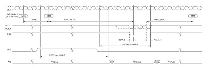
Note: 1.  $R_{TT(Park)}$  = Enable;  $R_{TT(NOM)}$  = Enable; WRITE preamble set =  $2^{t}CK$ ; and DLL = On.
