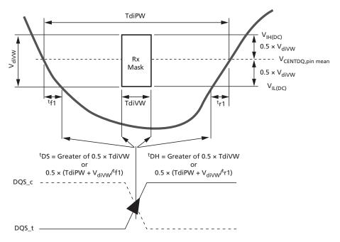
The following figure and table show an example of the worst case Rx mask required if the DQS and DQ pins do not have DRAM controller to DRAM write DQ training. The figure and table show that without DRAM write DQ training, the Rx mask would increase from 0.2UI to essentially 0.54UI. This would also be the minimum <sup>t</sup>DS and <sup>t</sup>DH required as well.
