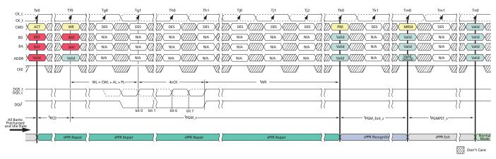
Table 44: DDR4 sPPR Timing Parameters DDR4-1600 through DDR4-3200
