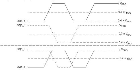
Resulting differential signal relevant for<sup>t</sup>RPST specification
