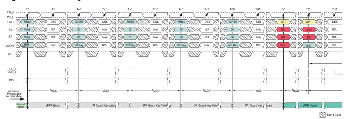
Figure 80: sPPR - Repair, and Exit
