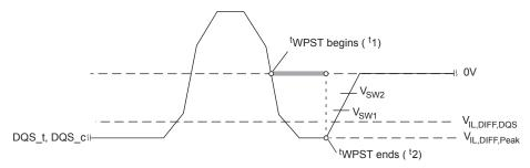
Notes: 1.  $V_{sw1} = (0.9) \times V_{IL,diff,DQS}$ .
