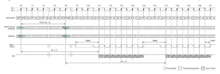
Notes: 1. BL8, AL = 0, CL = 11, Preamble =  $2^{t}$ CK,  $^{t}$ CCD\_S/L = 6. 2. DO n (or b) = data-out from column n (or column b).
