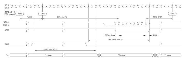
Note: 1.  $R_{TT(Park)} = Enable$ ;  $R_{TT(NOM)} = Enable$ ; WRITE preamble set =  $2^tCK$ ; and DLL = On.
