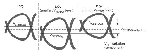
The following figure shows the Rx mask requirements both from a midpoint-to-midpoint reference (left side) and from an edge-to-edge reference. The intent is not to add any new requirement or specification between the two but rather how to convert the relationship between the two methodologies. The minimum data-eye shown in the composite view is not actually obtainable due to the minimum pulse width requirement.
