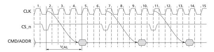
CAL gives the DRAM time to enable the command and address receivers before a command is issued. After the command and the address are latched, the receivers can be disabled if CS\_n returns to HIGH. For consecutive commands, the DRAM will keep the command and address input receivers enabled for the duration of the command sequence.
