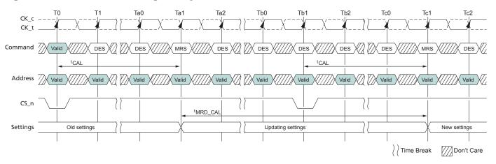
Note: 1. MRS at Ta1 may or may not modify CAL, <sup>t</sup>MRD\_CAL is computed based on new <sup>t</sup>CAL setting if modified.
