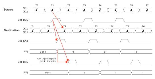
DQS driven by the controller during leveling mode must be terminated by the DRAM based on the ranks populated. Similarly, the DQ bus driven by the DRAM must also be terminated at the controller.
