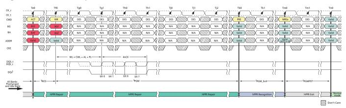
Table 41: DDR4 hPPR Timing Parameters DDR4-1600 through DDR4-3200
