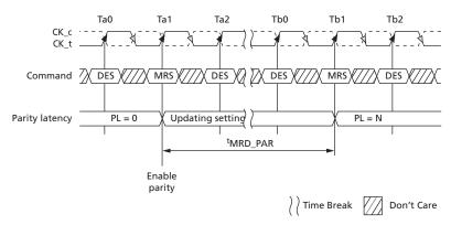
Note: 1.  ${}^{t}MRD_{PAR} = {}^{t}MOD + N$ ; where N is the programmed parity latency.
