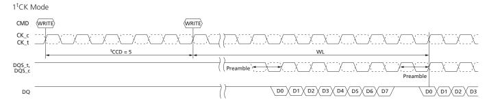
2<sup>t</sup>CK Mode: <sup>t</sup>CCD = 5 is not allowed in 2<sup>t</sup>CK mode.
