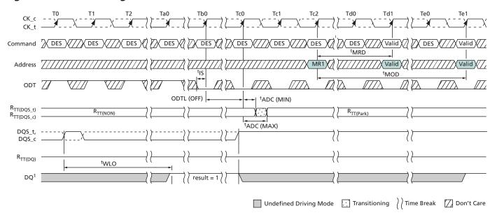
Notes: 1. The DQ result = 1 between Ta0 and Tc0 is a result of the DQS signals capturing CK\_t HIGH just after the T0 state.
