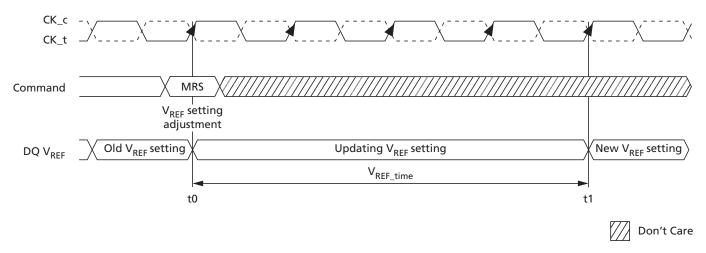
Note: 1. t0 is referenced to the MRS command clock t1 is referenced to V<sub>REE,tol</sub>
