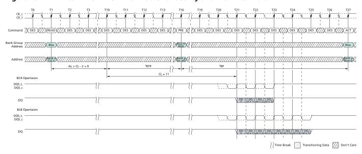
1. RL =20 (CL = 11, AL = CL - 2), Preamble =  $1^{t}$ CK,  $^{t}$ RTP = 6,  $^{t}$ RP = 11.
