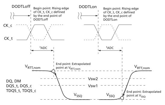
Figure 242: <sup>t</sup>ADC Definition with Dynamic ODT Control
