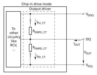
The output driver impedance,  $R_{ON}$ , is determined by the value of the external reference resistor  $R_{ZQ}$  as follows:  $R_{ON} = R_{ZQ}/7$ . This targets  $34\Omega$  with nominal  $R_{ZQ} = 240\Omega$ ; however, connectivity test mode uses uncalibrated drivers and only a maximum target is defined. Mismatch between pull up and pull down is undefined.
