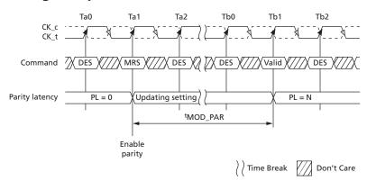
Note: 1. tMOD\_PAR = tMOD + N; where N is the programmed parity latency.
