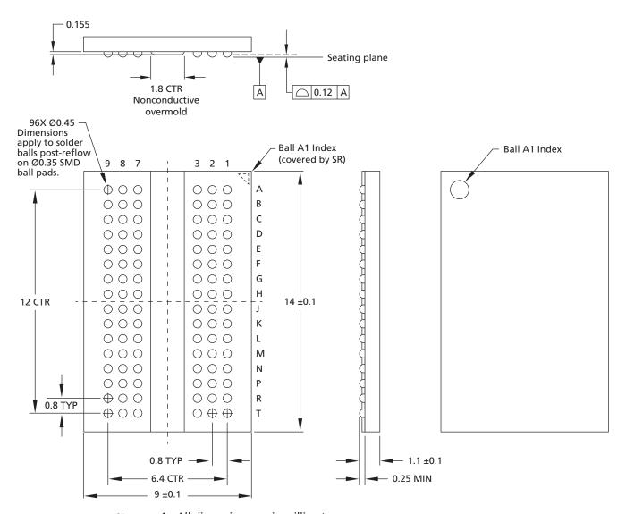
2. Solder ball material: SAC305 (Pb-free 96.5% Sn, 3% Ag, 0.5% Cu).
