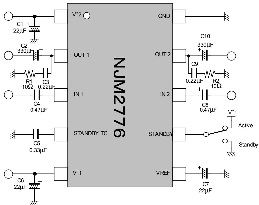
Note) Recommended the capacitors — C1, C3, C6 and C9 — are featuring higher frequency efficiency to prevent the oscillation.
