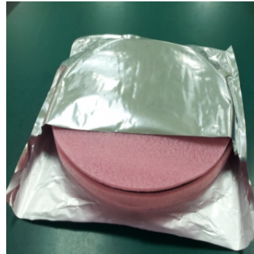
Sealed Moisture Barrier Bag (Foam Liner & Labels: ESD, MSL3, Caution, & Barcode)
