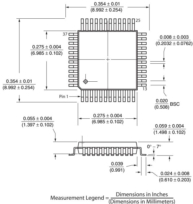
Measurement Legend =  $\frac{\text{Dimensions in Inches}}{\text{Dimensions in Millimeters}}$
