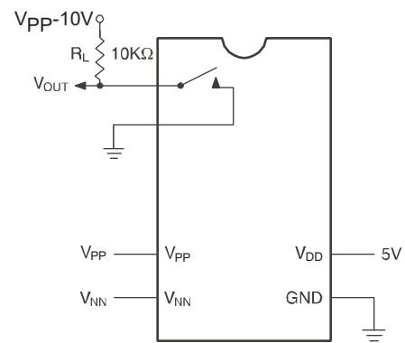
$T_{ON}/T_{OFF}$  Test Circuit
