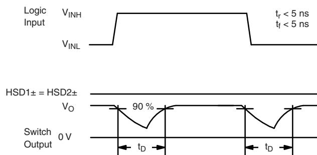
**Fig. 2 - Break-Before-Make Interval**
