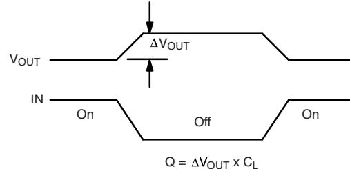
IN depends on switch configuration: input polarity determined by sense of switch.
