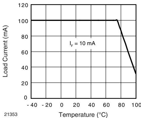
Fig. 1 - On-State Current (RMS) vs. Temperature
