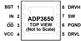
Figure 5. 8-Lead LFCSP Pin Configuration
