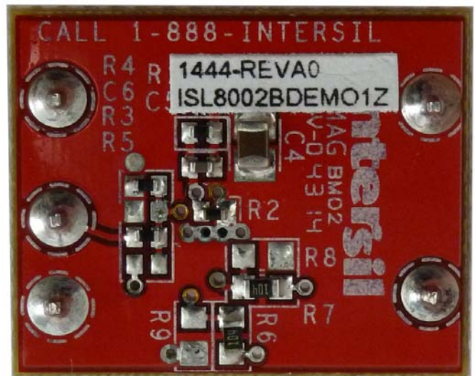
FIGURE 2. ISL8002BDEMO1Z BOTTOM SIDE
