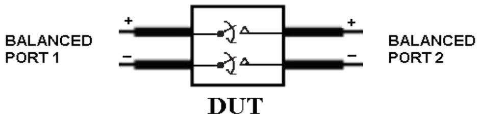
Differential Off Isolation Test Circuit
