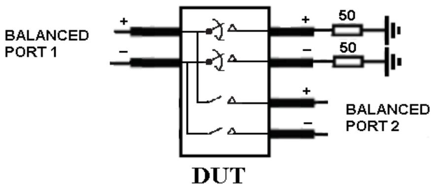
Differential Near End Crosstalk Test Circuit
