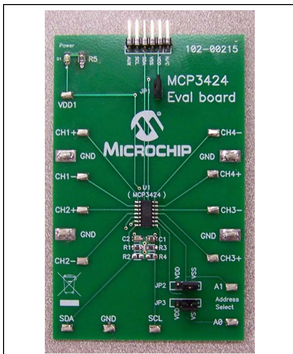
FIGURE 7-1: MCP3424 Evaluation Board.
