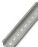
DIN rail, material: steel galvanized and passivated with a thick layer, perforated, height 7.5 mm, width 35 mm, length: 2000 mm
