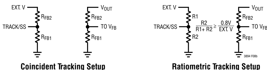
Figure 9(b): Setup for Ratiometric and Coincident Tracking
