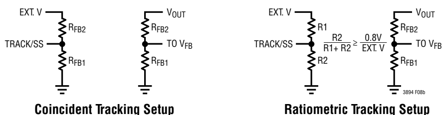
Figure 9(b): Setup for Ratiometric and Coincident Tracking
