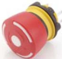
Emergency-stop non illuminated, plug-in terminals, twist release, 32mm diameter for 22.5mm mounting, foolproof to EN 60947-5-5, EN 418
