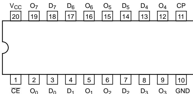
Figure 1. Pinout: 20-Lead Packages Conductors
