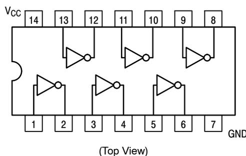
Figure 1. Pinout: 14-Lead Packages Conductors
