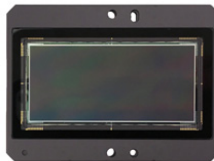
Figure 1. KAI-50140 CCD Image Sensor
