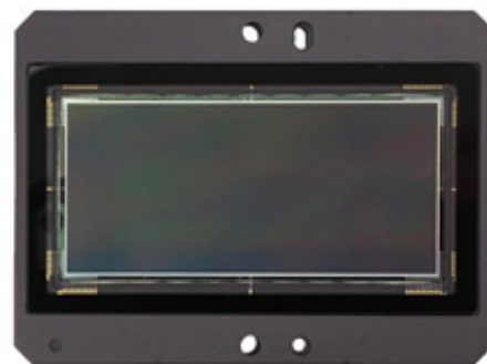
Figure 1. KAI-50140 CCD Image Sensor
