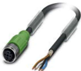
Sensor/actuator cable, 4-position, PUR halogen-free, black-gray RAL 7021, shielded, free cable end, on Socket straight M12, A-coded, cable length: 2 m, Shield not connected to knurl
