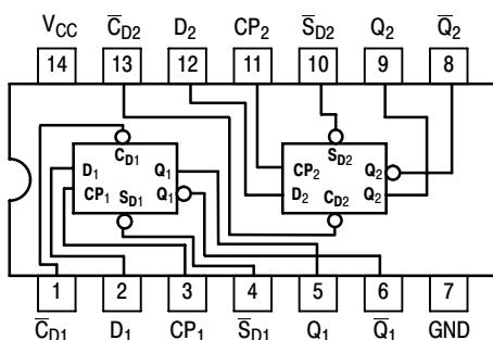
Figure 1. Pinout: 14-Lead Packages Conductors
