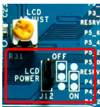
Figure 4-4 CY8CKIT-001 PSoC DVK LCD Power Jumper
