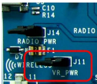
Figure 4-5 CY8CKIT-001 PSoC DVK VR_POWER Jumper
