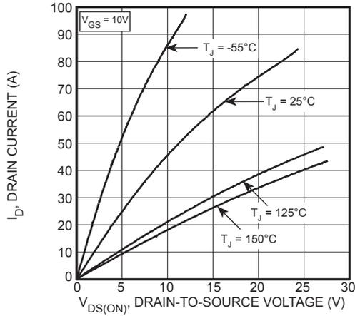
Figure 1, Output Characteristics
