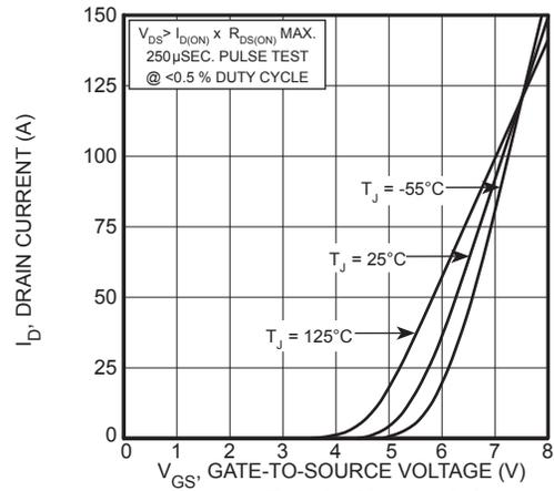
Figure 4, Transfer Characteristics
