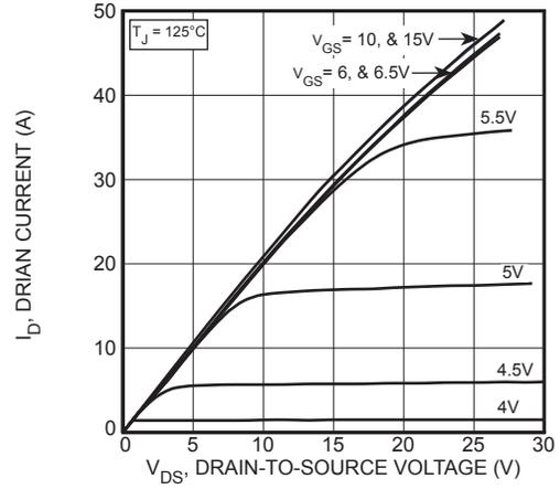
Figure 2, Output Characteristics
