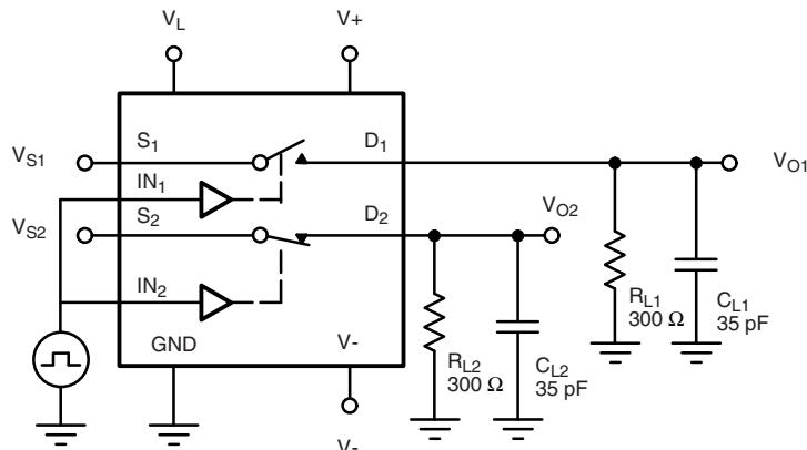
$C_L$  (includes fixture and stray capacitance)
