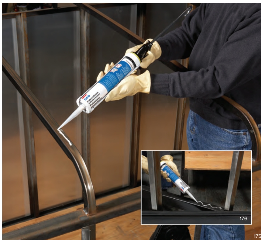
3M™ Polyurethane Sealant 560 moisture cures to a flexible seal/bond between exterior skins and metal framework and between wood flooring and metal framework. Tensile strength up to 580 psi is enough to replace mechanical fasteners in many situations.
