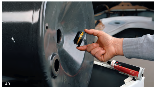
In washing machine repair, 3M™ Neoprene High Performance Rubber and Gasket Adhesive 1300 bonds with high immediate strength and seals the doughnut ring seal in the outer tub.
