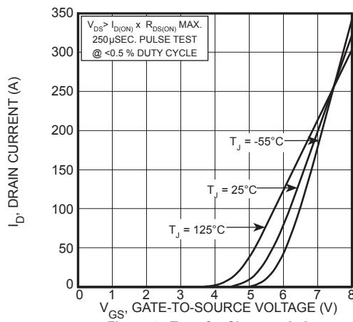
Figure 4, Transfer Characteristics
