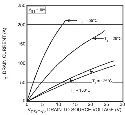
Figure 1, Output Characteristics
