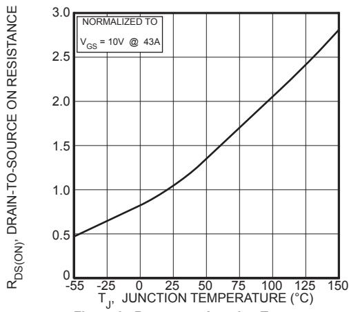
Figure 3,  $R_{DS(ON)}$  vs Junction Temperature
