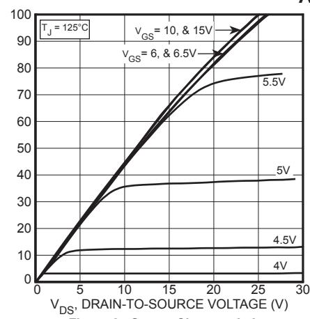
Figure 2, Output Characteristics
