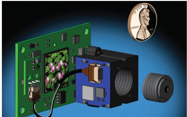
**SQUIGGLE RV motor and driver inside every M3-F module is the world's smallest linear motor system.**
