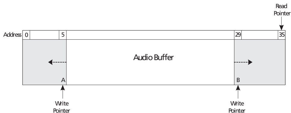
Figure 4-49: Audio Buffer Pointer Boundary Checking
