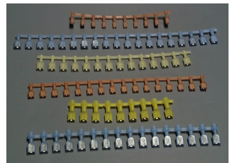
Quixon Fully-Insulated Quick-Disconnect Terminals (Red = 18 to 22 AWG; Blue = 14 to 16 AWG; Yellow = 10 to 12 AWG)
