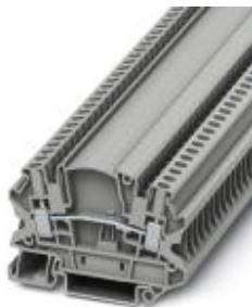
Feed-through terminal block, Connection method: Screw connection, Cross section: 0.14 mm<sup>2</sup> - 6 mm<sup>2</sup>, AWG: 26 - 10, Width: 6.2 mm, Color: gray, Mounting type: NS 35/7,5, NS 35/15
