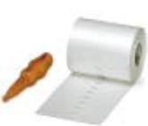
Marker for terminal blocks, Roll, white, Unlabeled, Can be labeled with: THERMOMARK ROLL, THERMOMARK X, THERMOMARK S1.1, Perforated, Mounting type: Snap into universal marker groove, Snap into flat marker groove, For terminal block width: 6.2 mm, Lettering field: 6.35 x 6.15 mm
