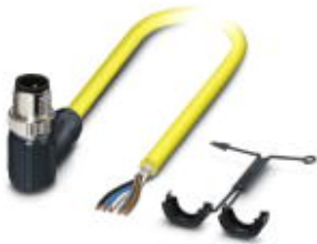
Sensor/Actuator cable, 5-position, PVC, yellow RAL 1021, shielded, Plug angled M12 SPEEDCON, A-coded, on free cable end, Cable length: 2 m
