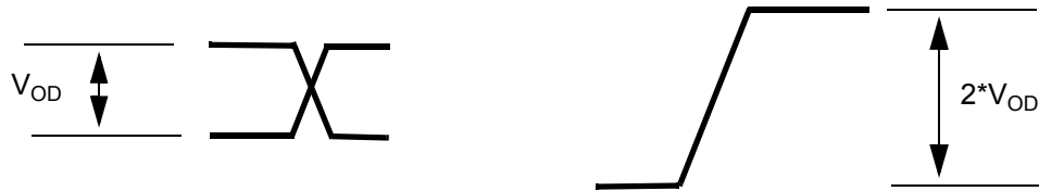
Figure 20 - Differential Voltage Parameter
