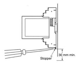
Mount the E5ZN at least 30 mm away from other devices to ensure easy mounting and dismounting.
