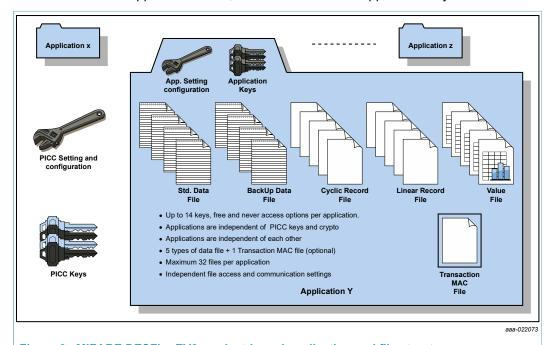
Figure 3. MIFARE DESFire EV2 product-based application and file structure
