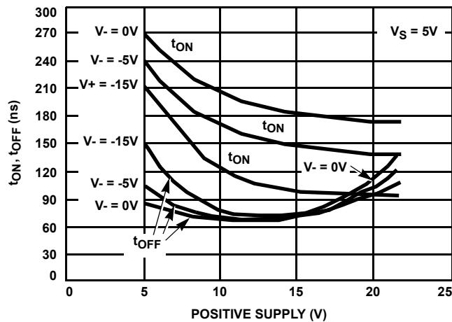
FIGURE 27. SWITCHING TIME vs POSITIVE SUPPLY VOLTAGE (NOTE 8)
