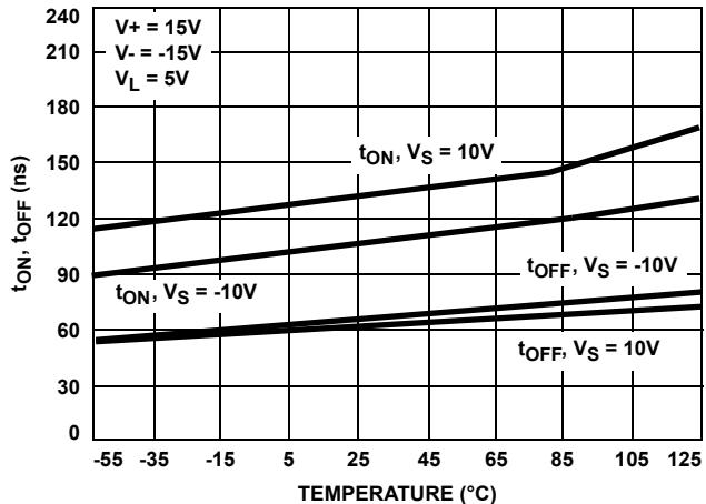
FIGURE 25. SWITCHING TIME vs TEMPERATURE (NOTE 8)
