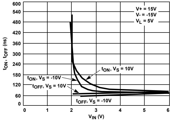
FIGURE 24. SWITCHING TIME vs INPUT LOGIC VOLTAGE (NOTE 8)
