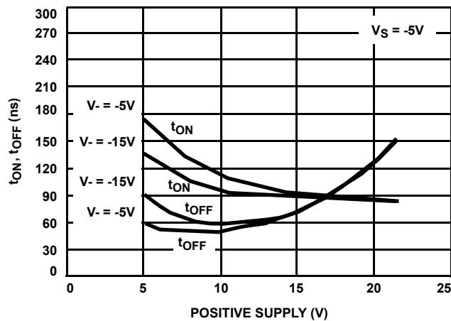
FIGURE 28. SWITCHING TIME vs POSITIVE SUPPLY VOLTAGE (NOTE 8)
