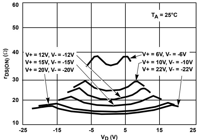
FIGURE 13.  $r_{DS(ON)}$  vs  $V_D$  AND POWER SUPPLY VOLTAGE
