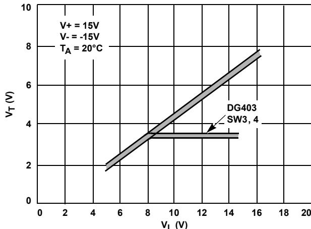
FIGURE 10. INPUT SWITCHING THRESHOLD vs LOGIC SUPPLY VOLTAGE
