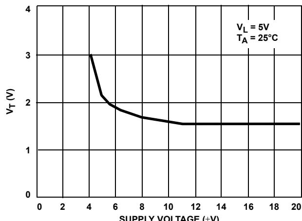
FIGURE 11. INPUT SWITCHING THRESHOLD vs POWER SUPPLY VOLTAGE
