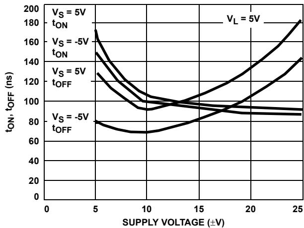
FIGURE 26. SWITCHING TIME vs POWER SUPPLY VOLTAGE (NOTE 8)
