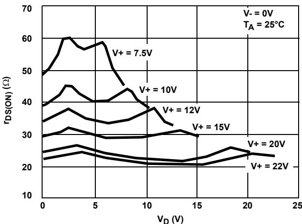
FIGURE 14.  $r_{DS(ON)}$  vs  $V_D$  AND SINGLE SUPPLY VOLTAGE
