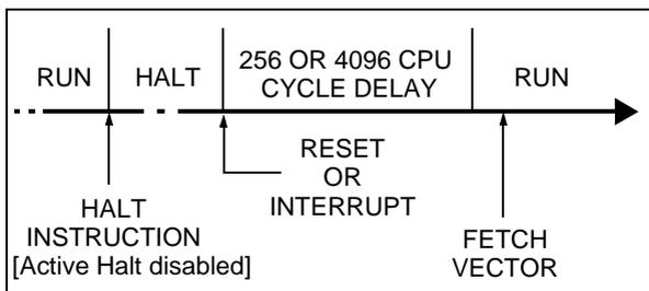
Figure 24. HALT Mode Flow-chart
