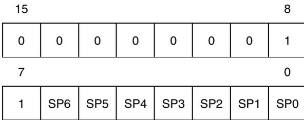
The Stack Pointer is a 16-bit register which is always pointing to the next free location in the stack. It is then decremented after data has been pushed onto the stack and incremented before data is popped from the stack (see Figure 10).
