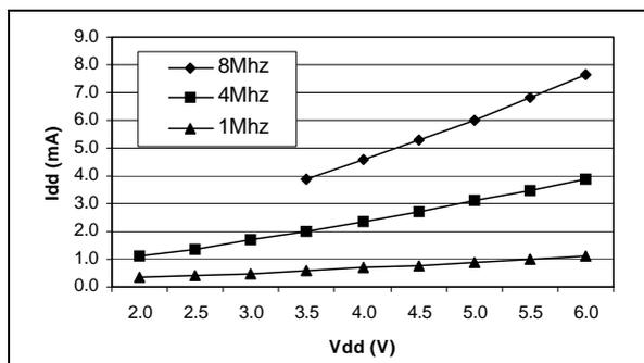
Figure 60. Typical  $I_{DD}$  in SLOW vs.  $f_{CPU}$
