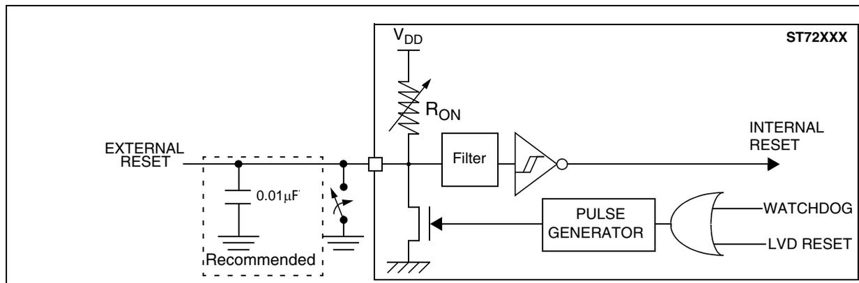
Figure 83.  $\overline{\text{RESET}}$  pin protection when LVD is disabled.<sup>1)2)3)</sup>
