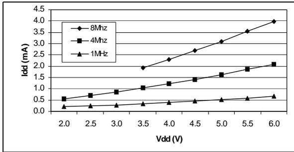
Figure 63. Typical  $I_{DD}$  in AWUFH mode at  $T_A=25^\circ C$
