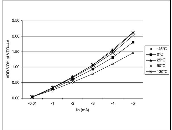
Figure 78. Typical  $V_{DD}-V_{OH}$  at  $V_{DD}=5V$
