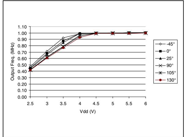
Figure 54. Typical RC oscillator Accuracy vs temperature @  $V_{DD}=5\text{V}$
