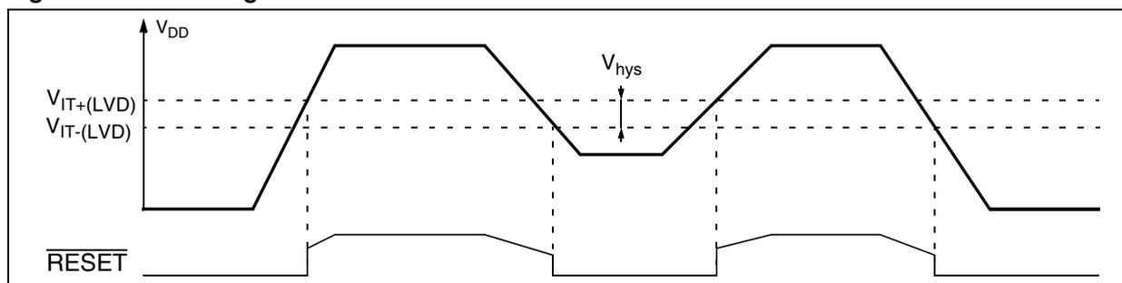
Figure 17. Reset and Supply Management Block Diagram
