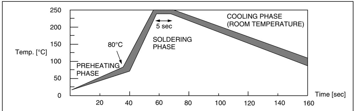
**Figure 92. Recommended Reflow Soldering Oven Profile (MID JEDEC)**
