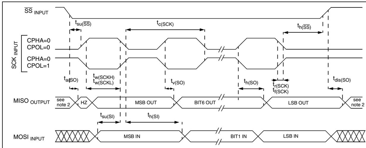
Figure 86. SPI Master Timing Diagram <sup>1)</sup>
