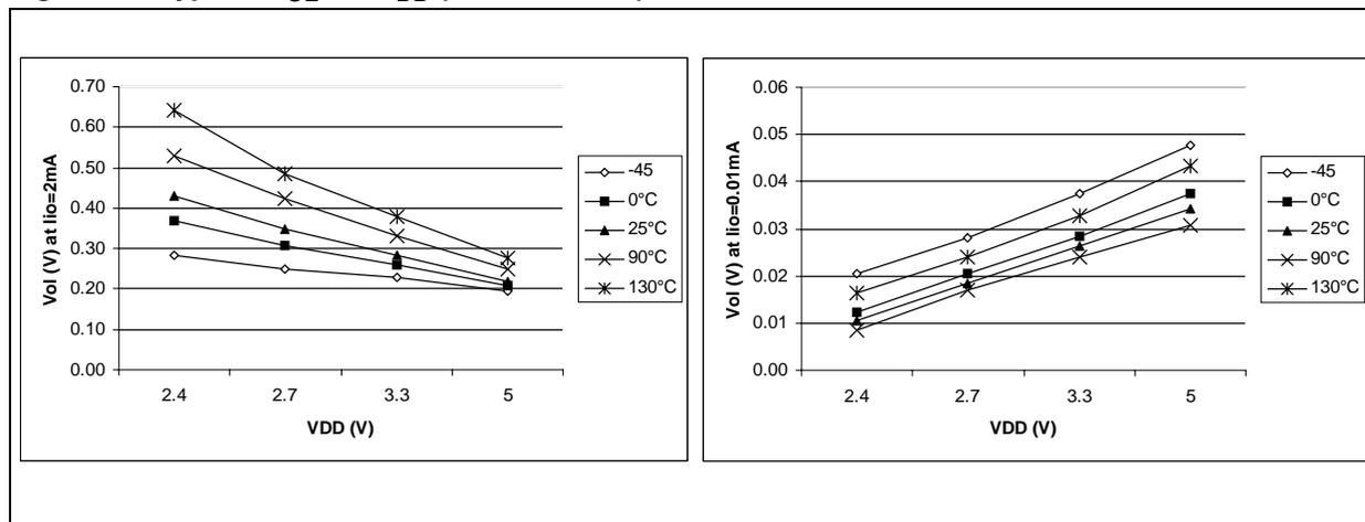
Figure 80. Typical  $V_{OL}$  vs.  $V_{DD}$  (high-sink I/Os)
