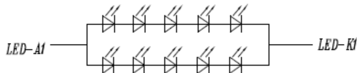
Figure: LED connection of backlight
