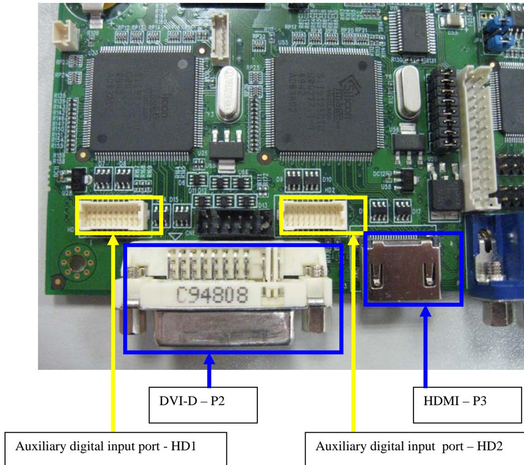
**(1) SGX-1920 without connect any I<sup>2</sup>C control on CN8 (i.e : HD-1000/-2000/-3000S/-3000)**
