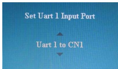
Set “Uart 1 to IP-50” : Enable Ethernet network (J1) support and disable second RS-232 serial control (CN1) support
